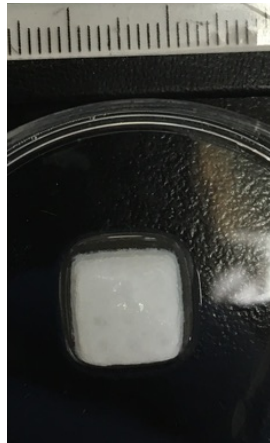
Compromised print resolution was observed when a gelatin slurry blended for 60 s was employed
