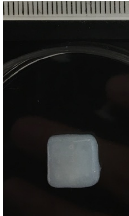
Compromised print resolution was observed when a gelatin slurry blended for 60 s was employed
