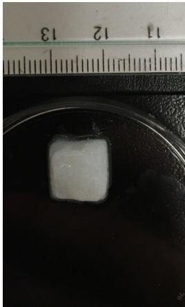
Compromised print resolution was observed when a gelatin slurry blended for 60 s was employed
